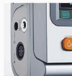
Standard interface for three parameters: FHR, FM, TOCO
